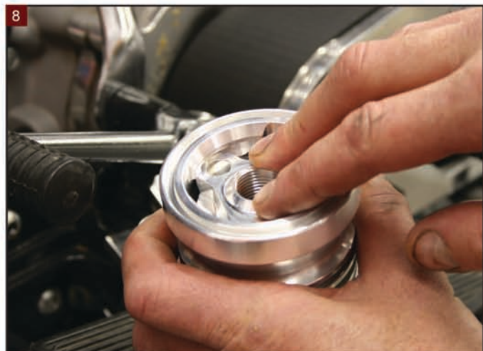
8 The filter element should slide easily into place on top of the bypass spring.
