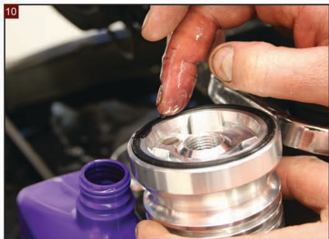
10 Lubricate the seal with a finger load of clean oil.
