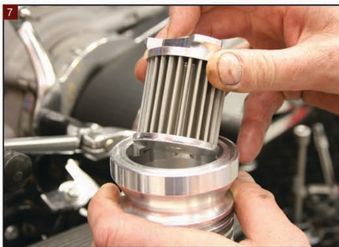
7 Next, install the filter element into the housing.
