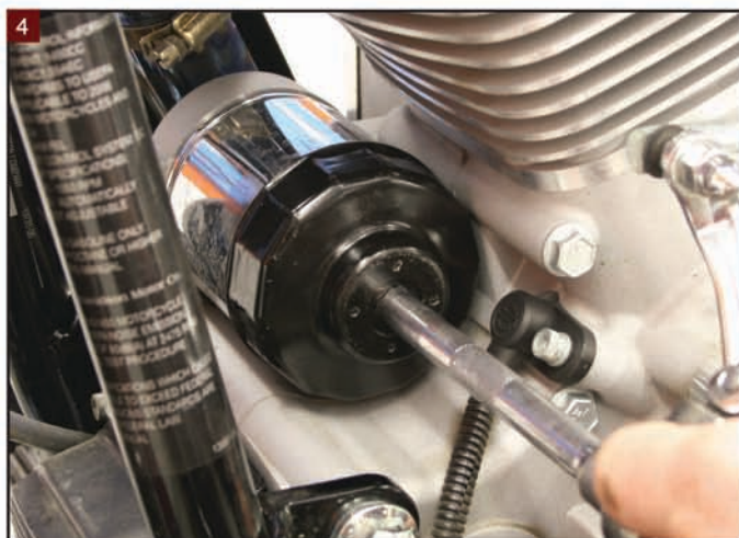
4 Loosen the oil filter using an oil filter wrench.
