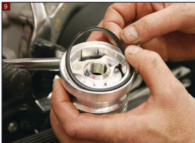
9 Slip the included oil seal into its slot in the housing.
