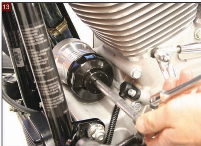
13 Use a wrench to tighten the filter until it is tight, then add an eighth of a turn.
