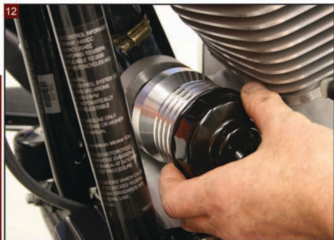
12 Thread the K&P housing onto the filter receptacle.
