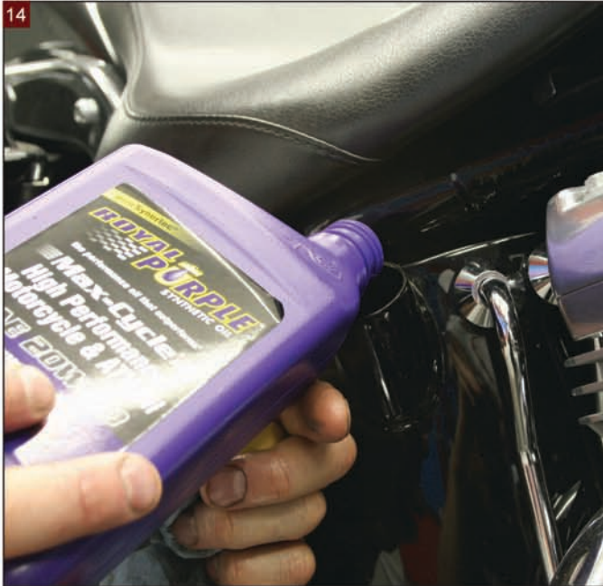
The oil of choice for the new filter is Royal Purple 20W-50.
