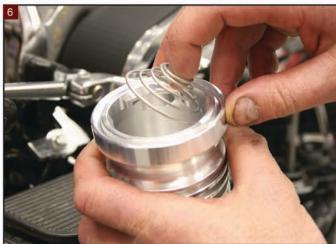
6 Install the bypass spring in the K&P filter housing.
