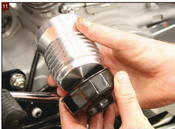
11 Slip the oil filter wrench onto the K&P filter housing.
